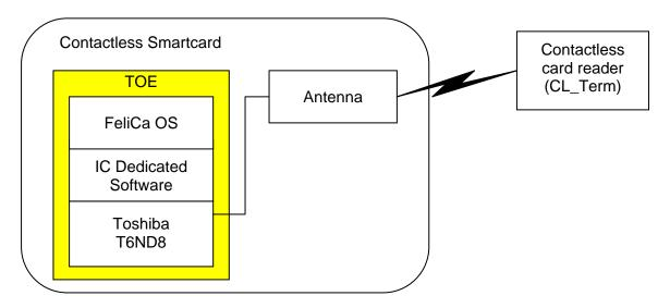
Figure 2: TOE physical scope
